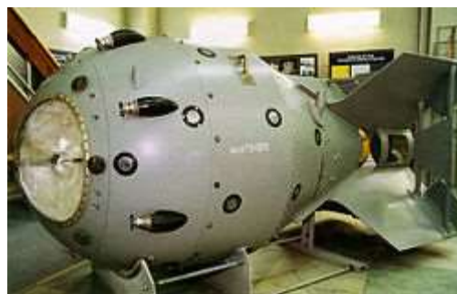
The first Soviet atomic bomb, "RDS-1", was an implosion type like the U.S. "Fat Man" bomb, even in appearance; the front "eyes" are radar fuses.
